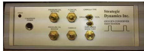
Figure 2. Oxygen Conserver Test System.
