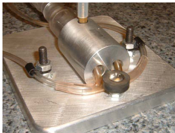
Figure 4. Artificial nose with nasal cannula.
